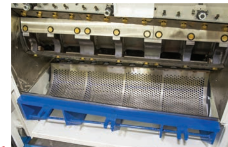
Screened Discharge Controls Particle Size
