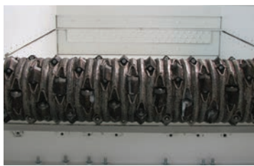
Patented U-Rotor and Feed Ram
