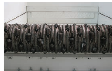
Patented U-Rotor and Feed Ram
