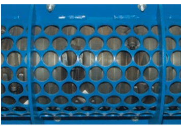
Screened Discharge Controls Particle Size
