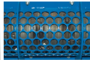
Screened Discharge Controls Particle Size
