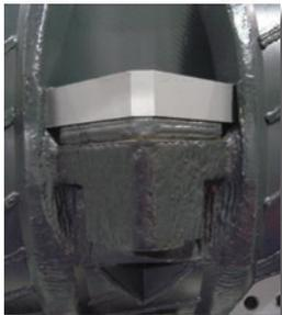
Unique in the industry, Vecoplan's replaceable cutter design minimizes downtime and maintenance costs. Cutters can be replaced or rotated by loosening two bolts. A complete cutting tool exchange can be performed in about two hours. Conventional shredders require extensive downtime, welding and maintenance expense just to maintain cutters.
