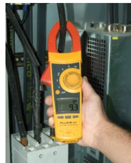
Actual Amp Load Measured Inside Panel with Amp Meter: 9.3
