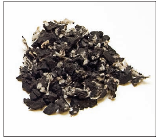
Re-Shredded Rubber from Secondary Shredder
