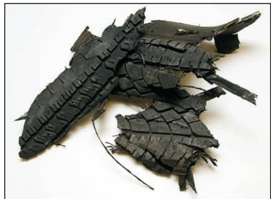
2" Shred Size with Steel Wire Still Present
