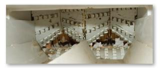
Unique infeed roller designs available, such as the above VTH 12-VU Paper Core Shredder, designed specifically for size reduction of paper cores.
