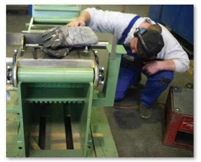
The Vecoplan VTH-VU Series horizontal shredders, or wood grinders as this industry has come to know them, are designed especially for size reduction of wood strips, edge rippings, slabs, and all long wood scrap, as well as lineal plastic scrap such as siding and vinyl window profiles.
