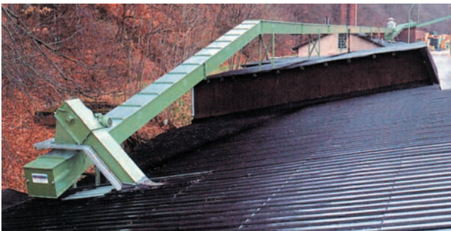
Drag Chain Conveyor installation for long distances.
