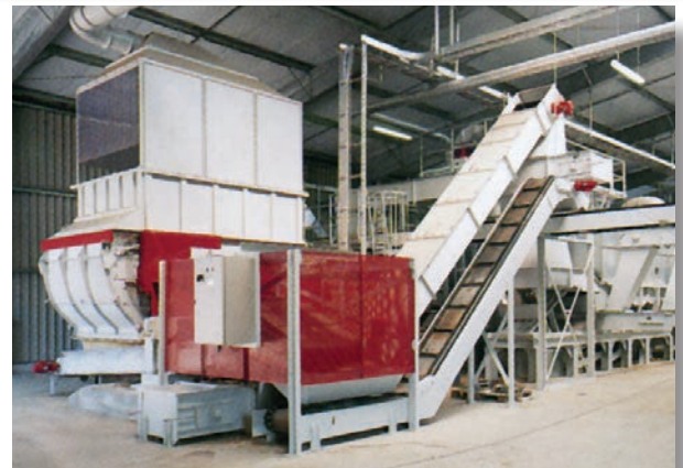
Drag Chain Conveyor installation for steep inclines.
