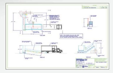
Designed specifically to deliver a quick, easy, and affordable solution for the unloading of shredding trucks, Vecoplan offers a variety of options that enable TUCS<sup>™</sup> to be custom tailored to fit your particular operations. These include a true dump & run conveying system for the absolute fastest truck unloading, a floor mounted conveyor for metered feed, and a below floor level conveyor for plants that employ pits.
