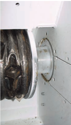
Double Side Walls and Easy Access to Wear Items Reduces Maintenance Costs
