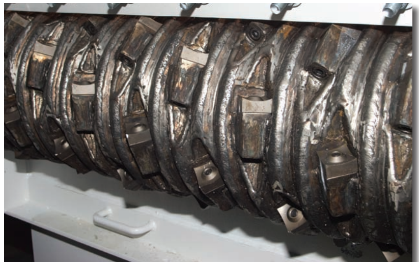
Hard-Faced Rotor for Exceptional Wear Characteristics
