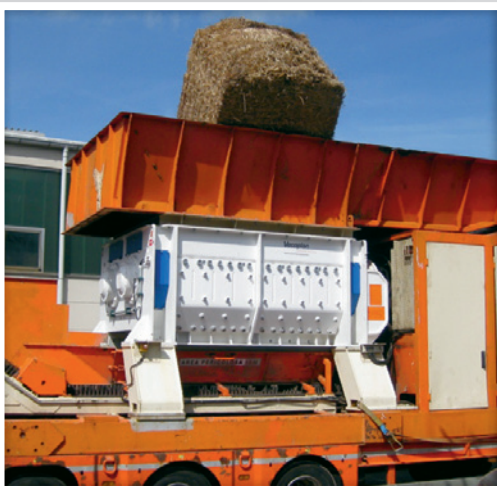
Example: Double-shaft shredder (WZ)
