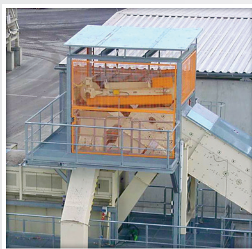
Example: Overbelt magnetic separator (VÜB)
