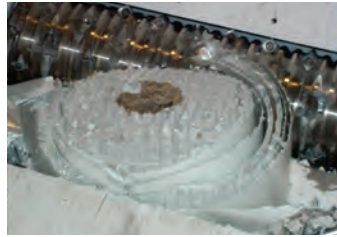
...Process Ram feeds material into Cutting Rotor...
