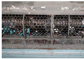
...Screened Discharge Regulates Particle Size...
