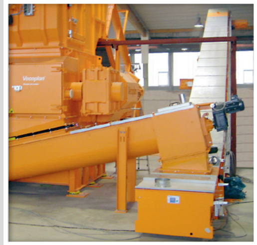
Example: Screw conveyor and drag chain conveyor
