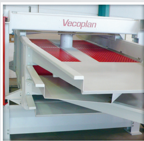
Example: Oscillation screen (VSS)
