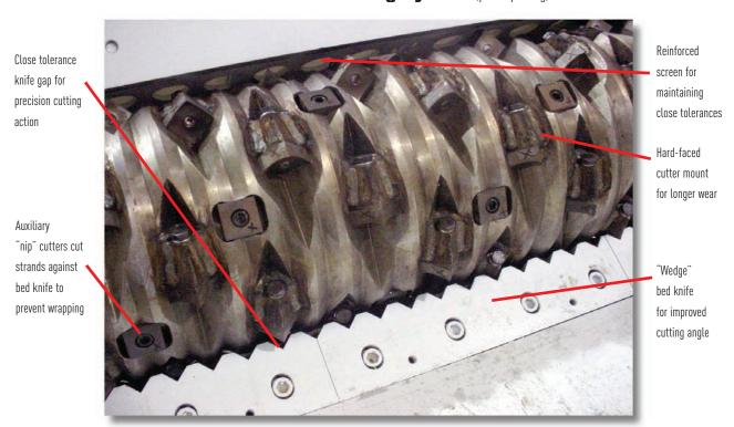
A revolutionary design which eliminates the typical difficulties usually associated with the processing of plastic film and synthetic fiber materials.
