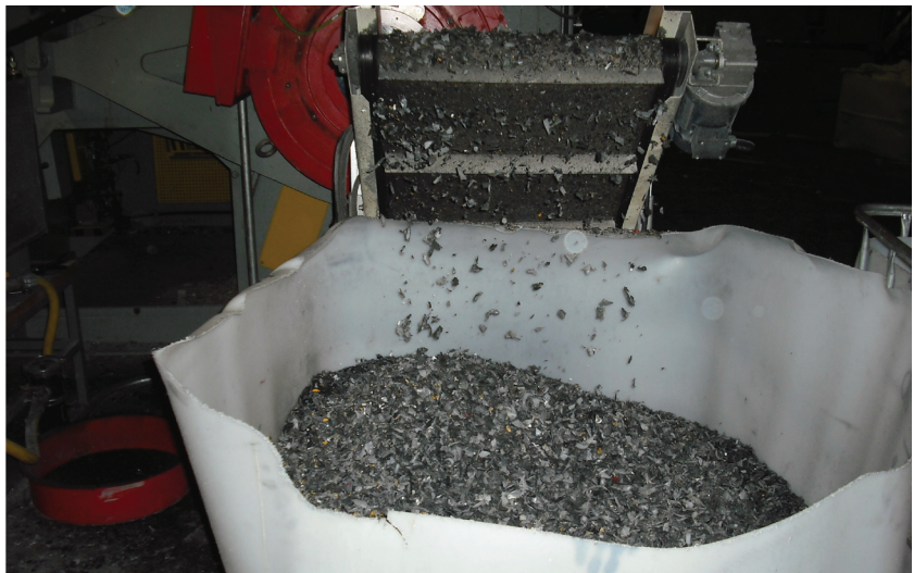
Discharge from RG70/200-XL Shredder
