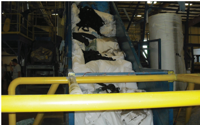
Material on infeed conveyor feeding RG70-FF-HT Shredder
