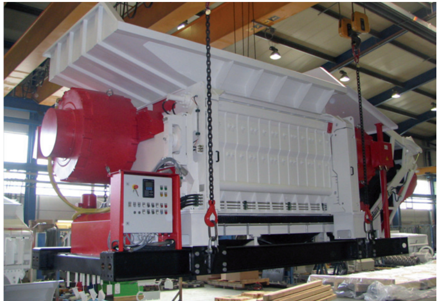
New pre-shredder, type VVZ 250 T „Hurricane“ with HiTorc drive
