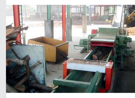
The drum chipper is feed by a dosing conveyor with following vibratory conveyor. In front of the drum chipper a metal detector is installed. On the occasion of the take over test
